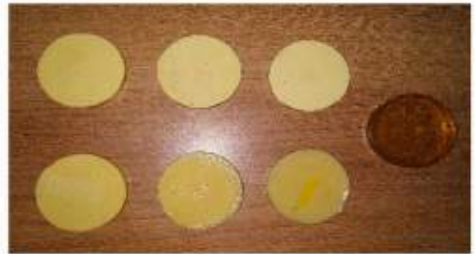
Fig. 1. Pictures of prepared \text{Bi}_2\text{O}_3 /UPR composite samples for different filler wt %.
